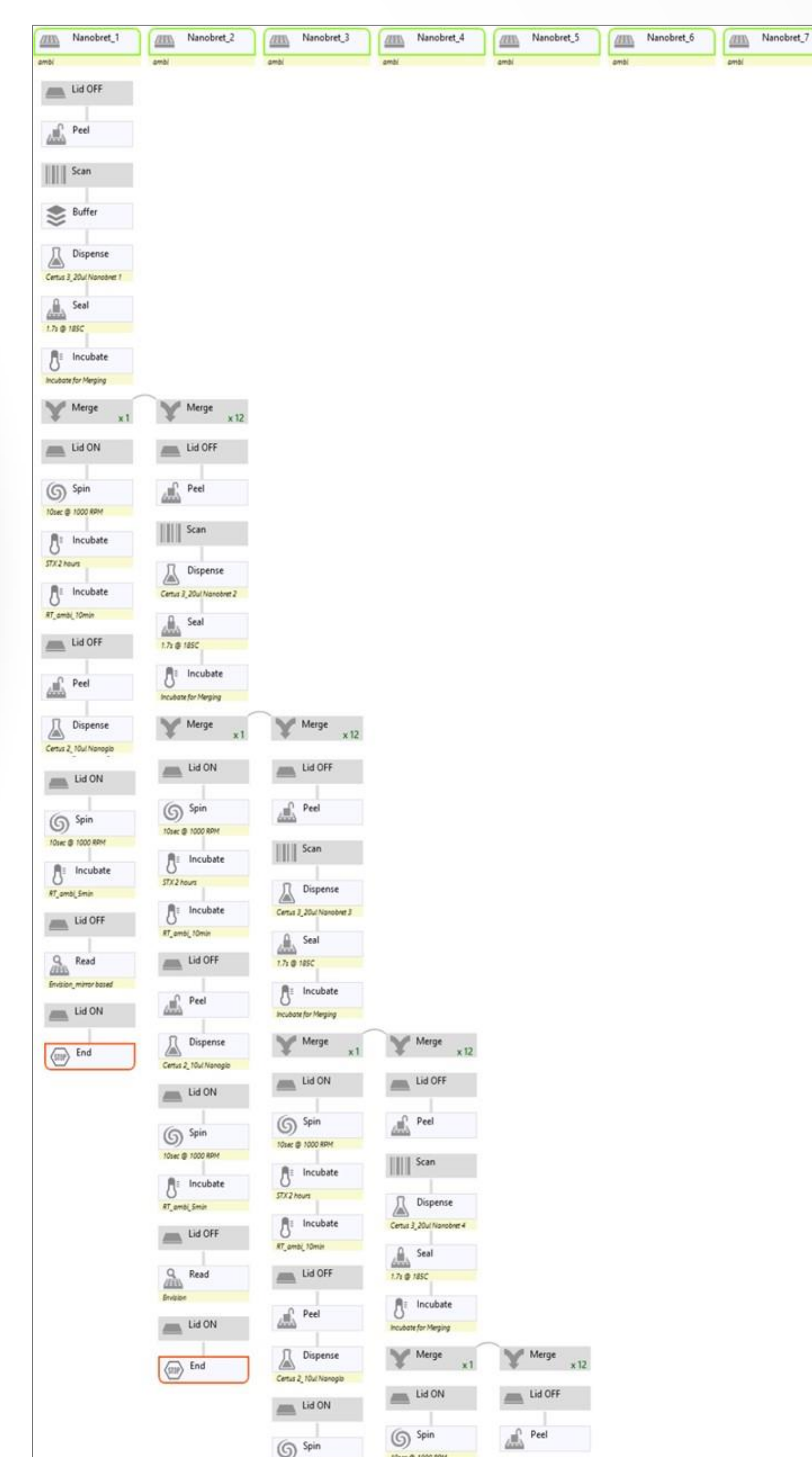
Figure 1: Example of a multiple protocol thread strategy within a workflow that allows multiple assay plates to be run simultaneously.
